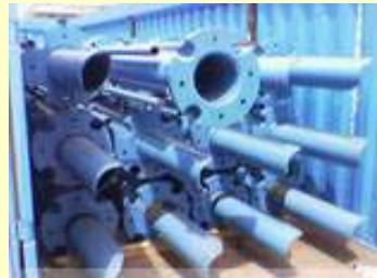
Flanged string of 10" Pipe fitted with two 2" water jet lines and a 2" compressed air line
