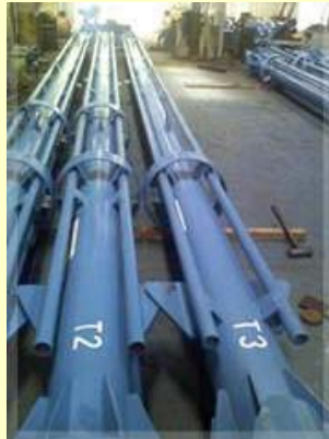
Flanged string of 10" Pipe fitted with two 2" water jet lines and a 2" compressed air line
